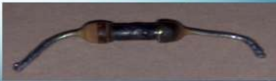
Physical appearance of bad/defective resistor
